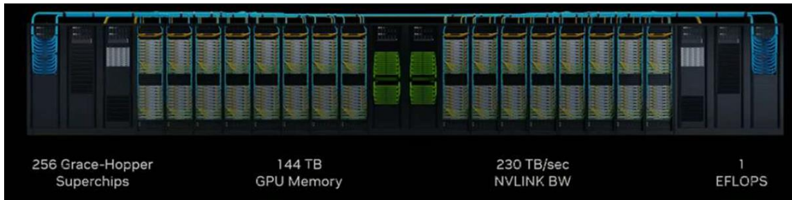
Figure 3 Representation of a large AI/ML cluster. In blue, the Front End Interconnect (FEI). In green, the Back End Interconnect (BEI). [6]
