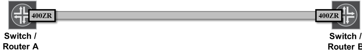
Figure 6: Router/Switch line card with 400ZR unamplified point-to-point interface
