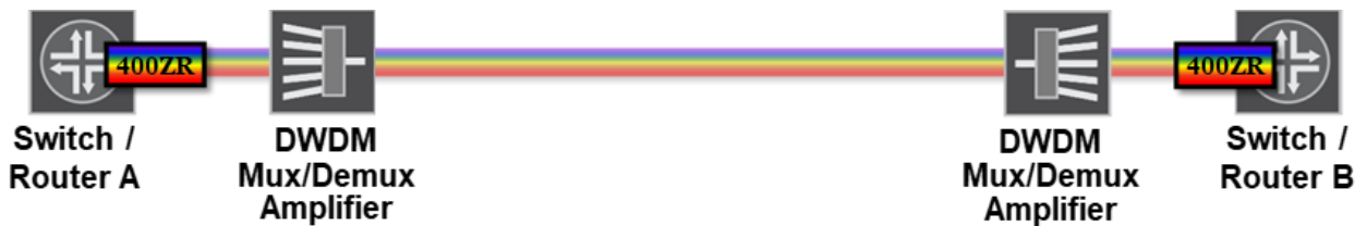
Figure 3: Switch/Router line card with 400ZR DWDM interfaces
