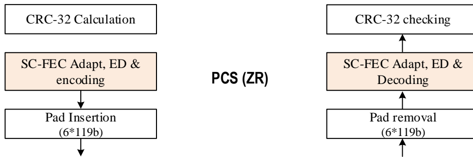
Figure 26: 400ZR HD-FEC processes
